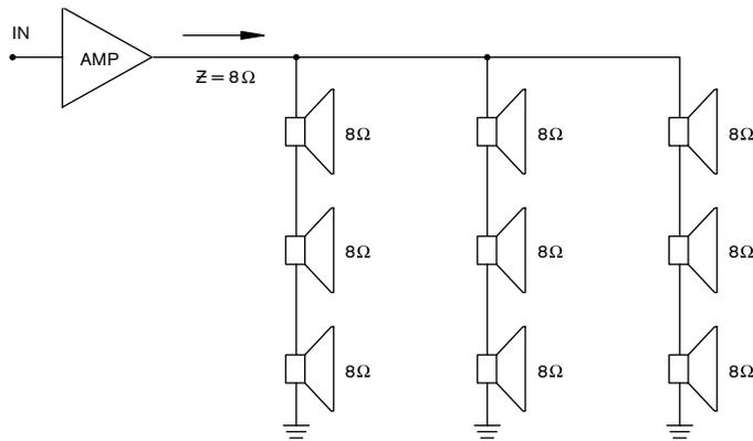
Figure 1. Low-Impedance Series-Parallel 8 ohm Direct Drive Constant-Voltage-2
