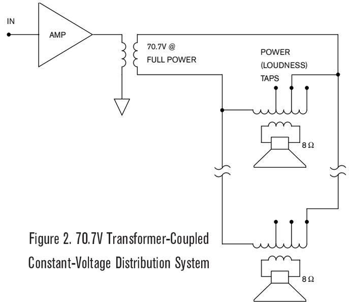
Figure 2. 70.7V Transformer-Coupled Constant-Voltage Distribution System
