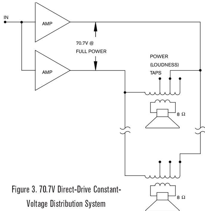
Figure 3. 70.7V Direct-Drive Constant-Voltage Distribution System
