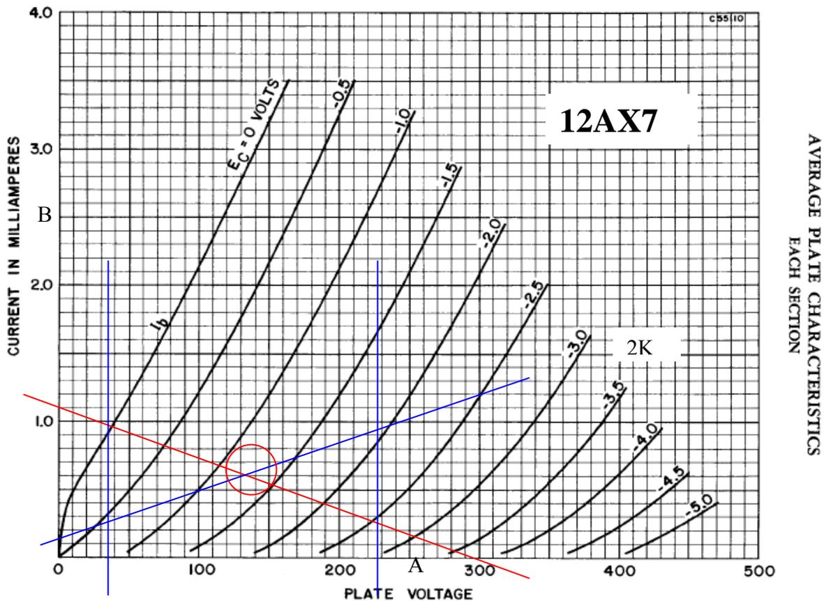
However the two 12AX7 halves have a common cathode resistance, bypassed, which I think provides a level of NFB. The second half also has NFB from plate to grid via a 4M7 resistor. above. Need to do a simulation.
